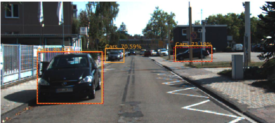
Figure 1.1: Object detector predicting the position of cars in a real-world environment, in red is represented the objects ground truth and in orange the predictions.
